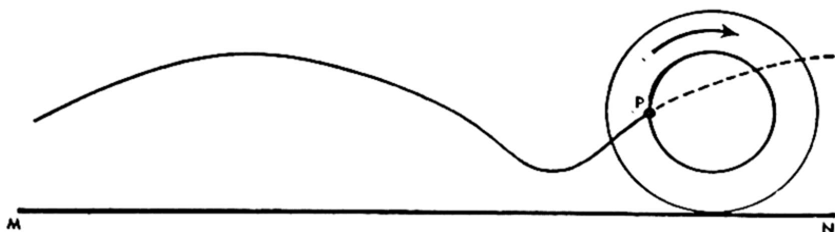
FIG. 67.—The prolate cycloid is generated by the point P on the smaller circle as the larger circle rolls along the line MN .
