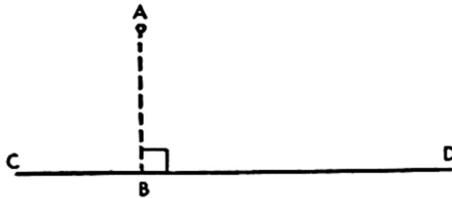
FIG. 43.—Through the point A one and only one perpendicular can be drawn to CD .
